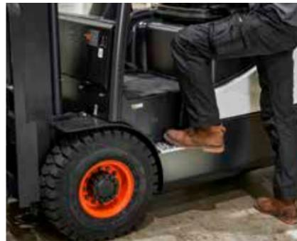
This forklift features a low step height, facilitating easy and safe operator entry and exit, complemented by an easy entry grab bar and an anti-slip step plate.
