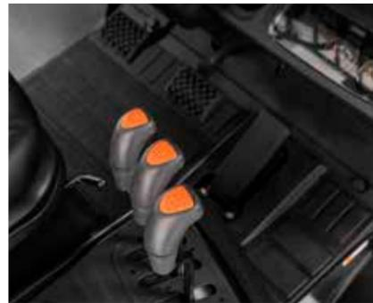
Effortlessly control with automotive-style pedals—large accelerator, inching, and air-boosted power brake. Brake with ease, even when the engine is off, thanks to the spring-actuated parking brake handle.
